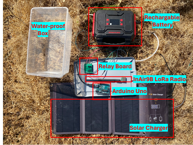
Figure 3.13: The illustration of the solar-powered sensor node.
