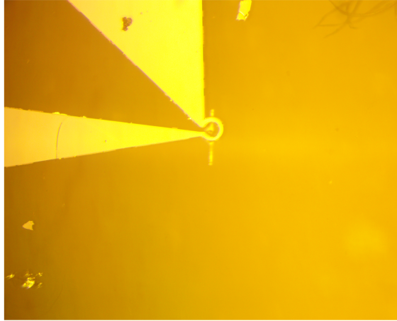
Figure 6.7: Optical microscopy image of Cr 2 O 3 micro-structure device integrated on the micro-coil of the non-superconducting omega-shaped planar micro resonator.
