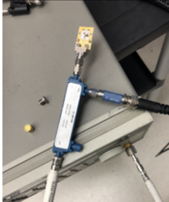
Figure 6.5: Measurement setup to characterize the eigen-frequency of omega shaped planar micro-resonator.
