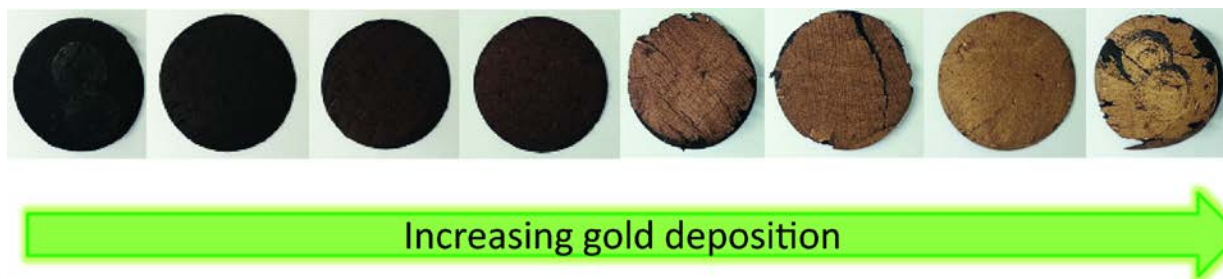
Figure 3.5 Increasing the gold sputter deposition time gives an air-FCG electrode with more gold visible on the electrode surface.
