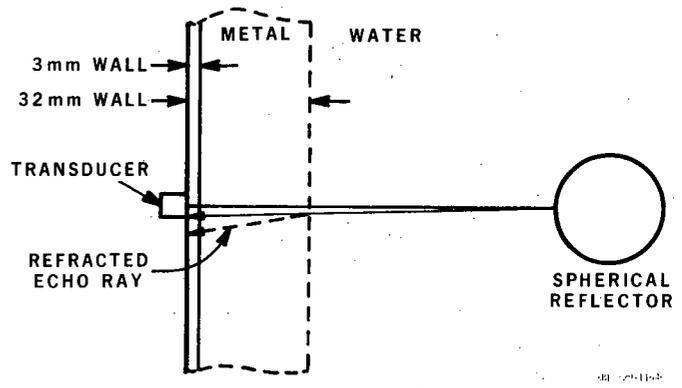
Fig. 4 Illustration of the effect of wall thickness on the echo signal from a spherical reflector. For a thick wall (shown dotted), the echo signal is spread over a larger area due to refraction effects at the water-metal interface.
