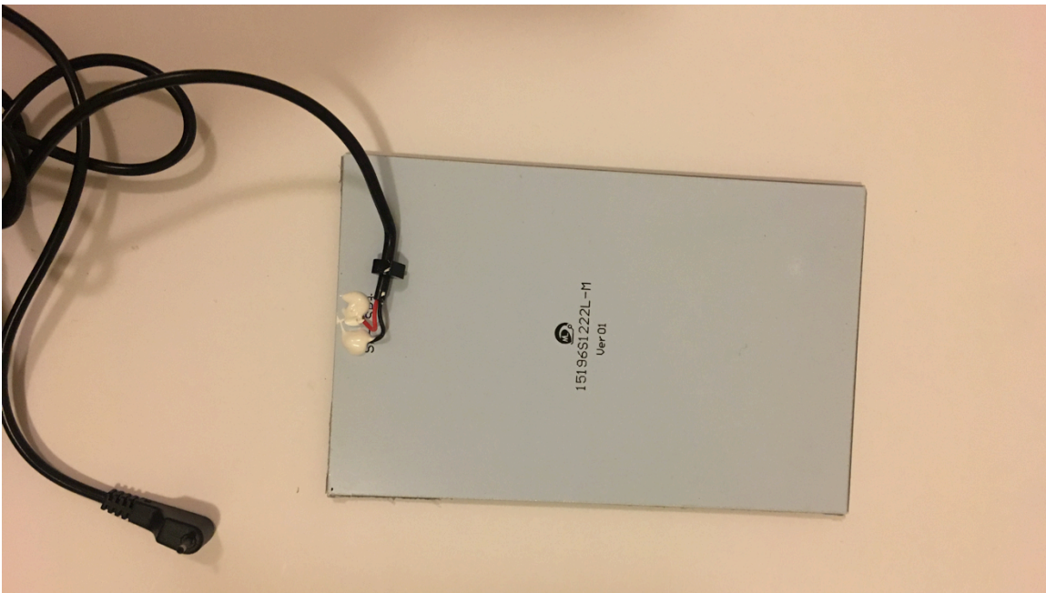
Figure 30: Example of Weak Connection Point
