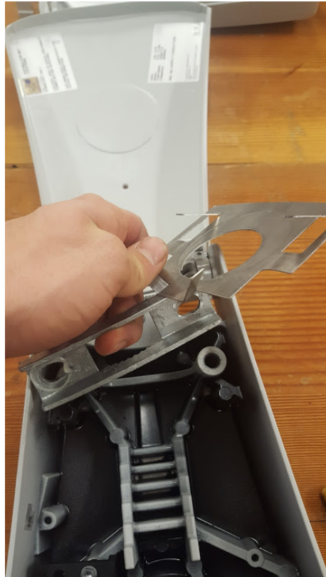
Figure 39: SL 2 Design standardization for metal components could increase to promote remanufacturing potential
