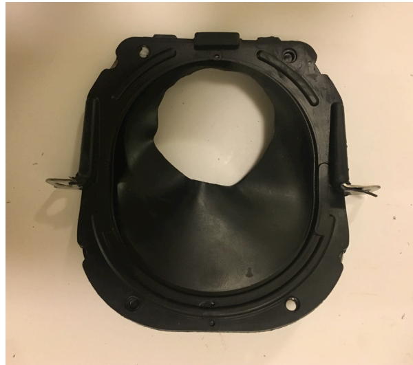
Figure 41: SL 3 adaptor example of mixed materials
