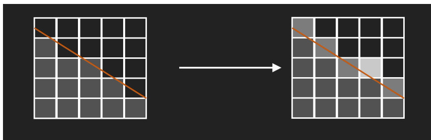
Figure 3.5: Steps involved in MLAA: 1) finding separation lines (top left) 2) computing the area of influence for each lines (bottom) 3) blending colors of opposite pixels (top right)
