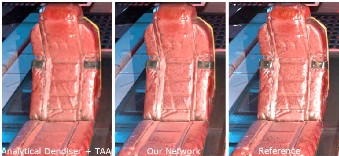
Figure 4.32: Our network is able to create complex filters that can retain high frequency detail giving a more sharper look (middle) than the analytical denoisers(left). Our results are comparable to the high ray count reference (right).
