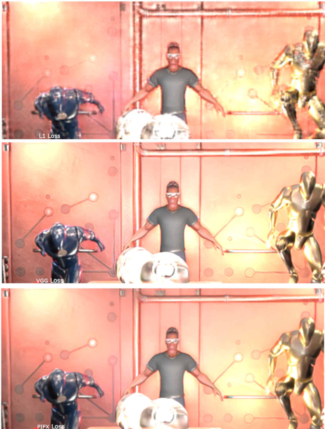
Figure 4.12: Comparison showing results from training using different loss functions. PIFX loss is able to produce sharp images without pattern artifacts
