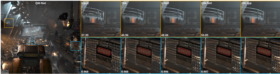
Figure 3.1: A comparison of different reconstruction techniques on a frame from the INFILTRATOR scene with PSNR (top row) and SSIM (bottom row) metrics. TAA has the worst reconstruction quality with excessive blurring followed by direct prediction with U-Net. QW-Net (ours) produces the best results with quality comparable to brute force sampling with 256 samples per pixel.
