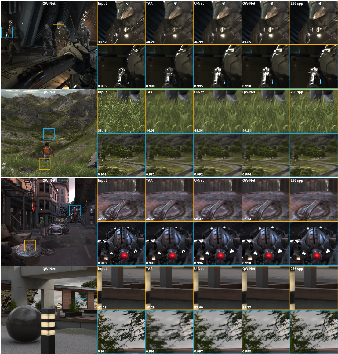
Figure 3.13: Representative frames from our test datasets. We compare the visual quality of TAA, U-Net, and QW-Net (INT4), compared to the 256\times supersampled reference. For each frame we magnify two areas of interests for easier comparison. We also show the PSNR metrics in the upper comparison rows and the SSIM values in the lower rows. TAA produces significantly lower metrics for all test frames, losing sharpness, and sometimes producing noticeable ghosting (e.g. ZENGARDEN, top row). U-Net closely approximates the reference, but is also consistently below QW-Net in quality metrics, and sometimes produces color shifts (e.g. INFILTRATOR, bottom row).
