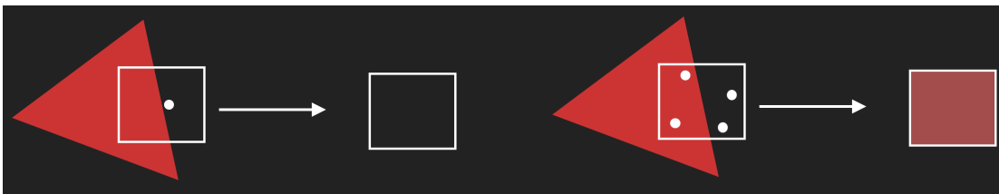
Figure 3.4: Sampling a triangle with 1 sample per pixel (left) and 4 samples per pixel with MSAA (right)
