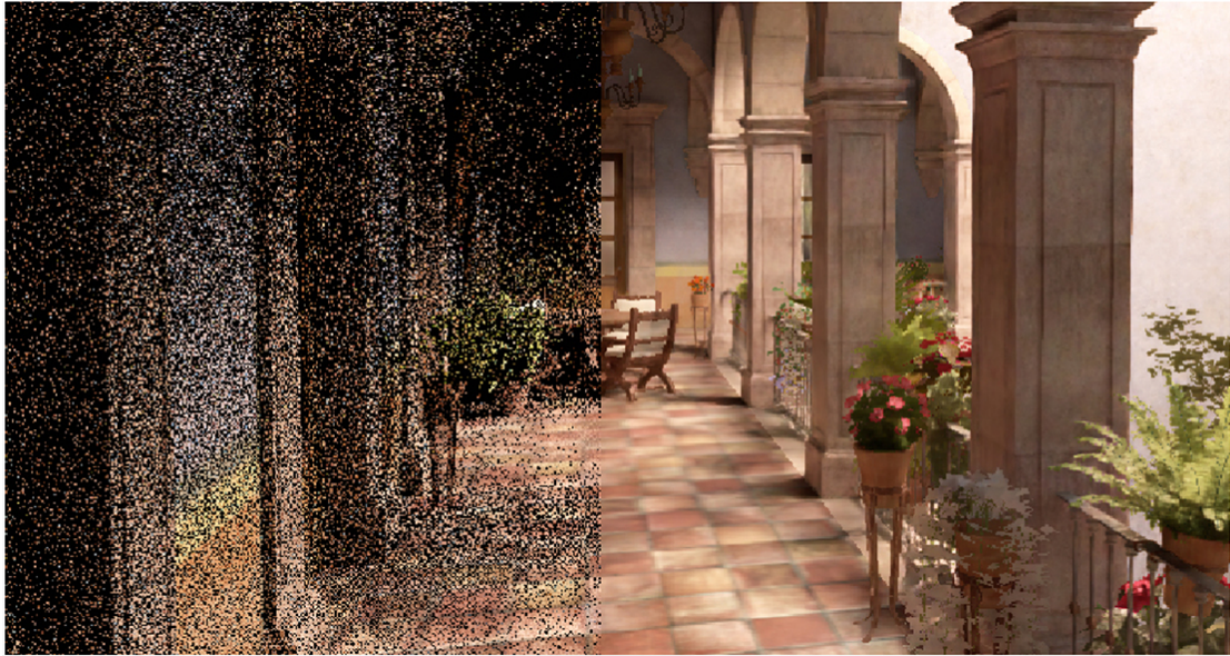
Figure 4.5: The input (left) and output(right) from a recurrent autoencoder based denoiser
