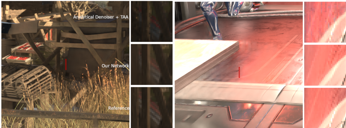
Figure 4.28: Time slice shown for a small segment in Dock and Scifi scene. Our network produce a smoother result while analytical solution contains discontinuities.
