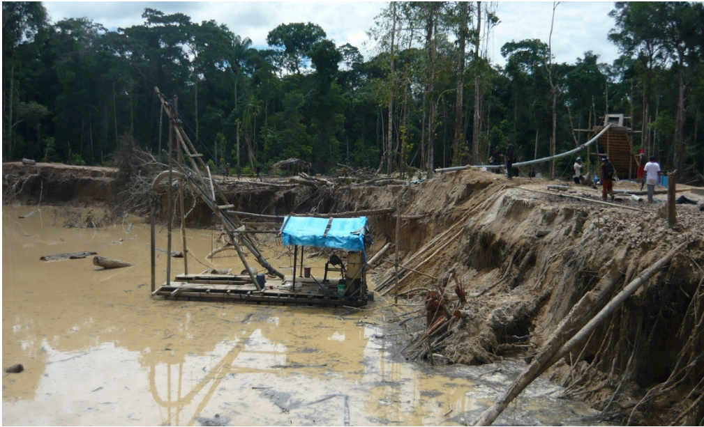
Figure 32: “La Chupadera” (The Sucker) Floating from a Raft, the Snout of the Tube Sucks the Sediment From the Watery Pit Photo shown with permission of Edgar Estumbelo
