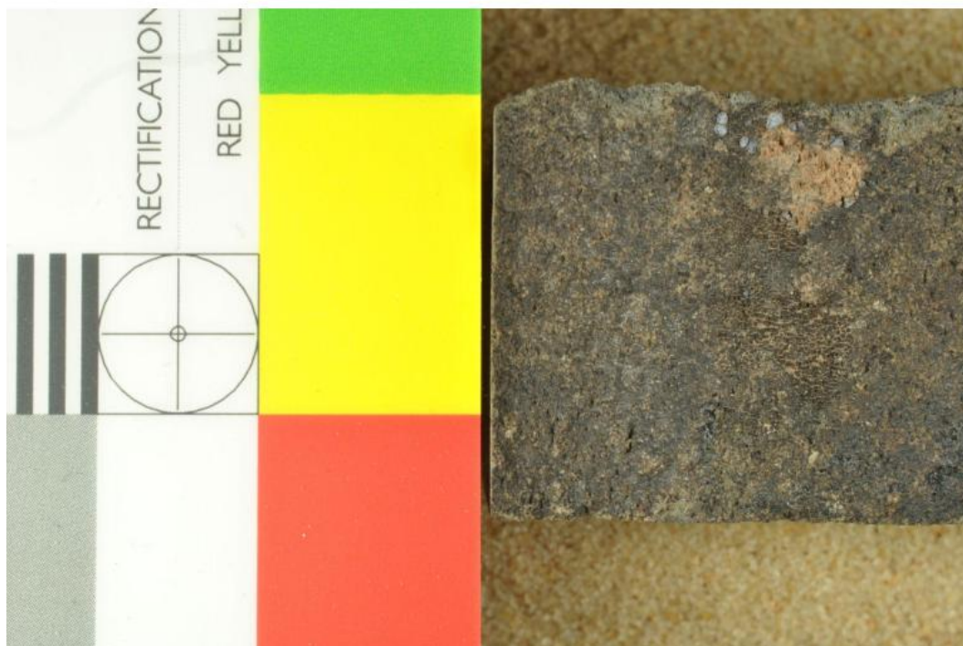
Figure 5.23 – Cross section and plan view of AB1DM5U1L2F-B. Top: Cross section of heat affected surface. A small orange rind is seen on the edge closest to the color scale. Bottom: Plain view of the heat affected surface. (Photo courtesy by Eric Blinman)
