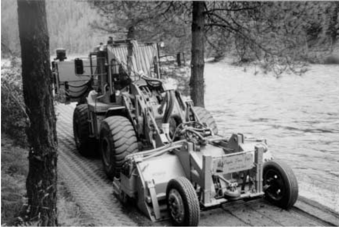
Fig. 3. Mobile In Place Processor mounted on a "Cat" loader - rotary drum on front lift arms and power pack at rear.
