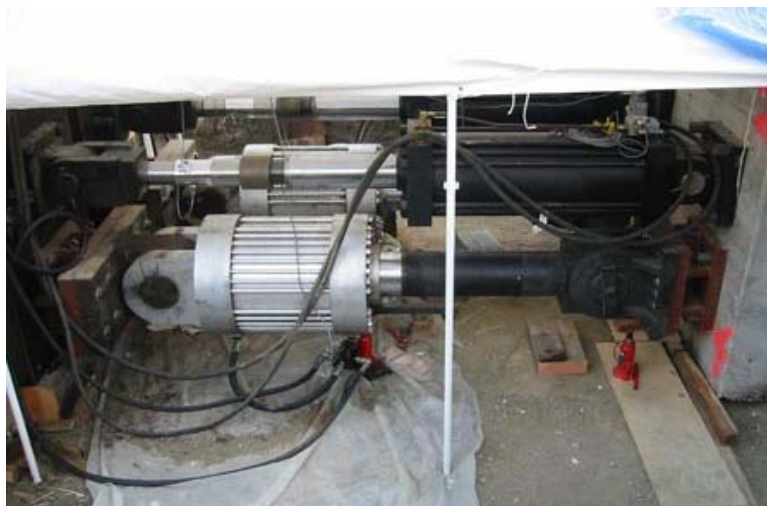
Figure 2.19. Fixed-head test actuator configuration
