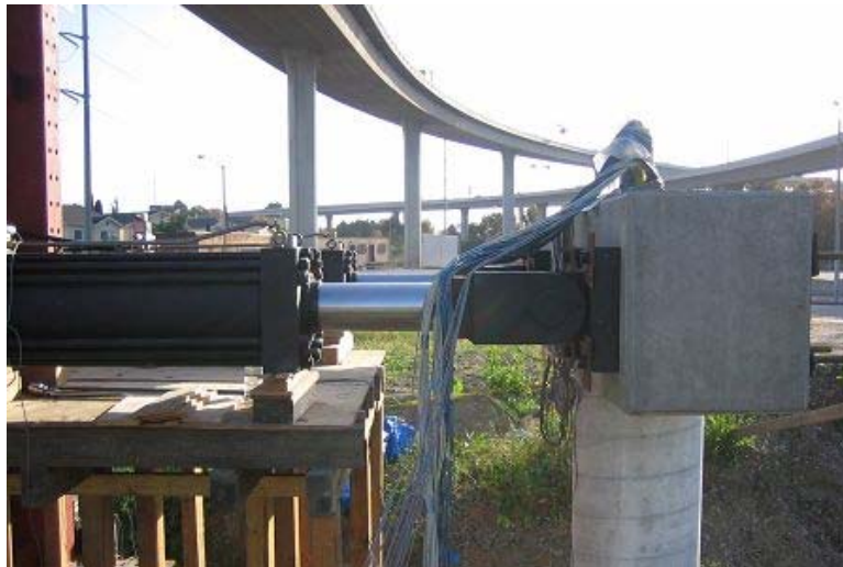
Figure 2.18. Flagpole test actuator configuration
