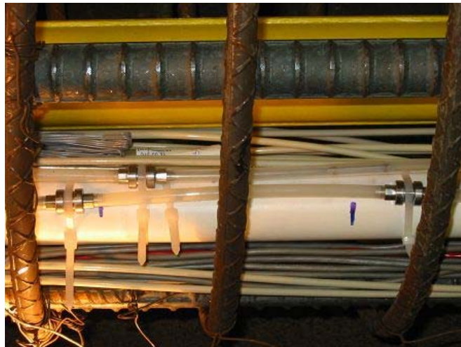
Figure 2.12. FGB housings and anchors shown installed on LVDT housings installed in flagpole specimen.
