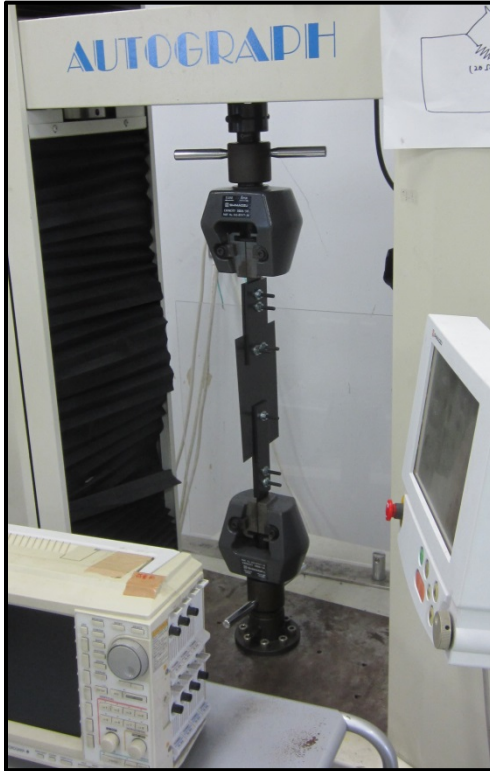
Figure 34 - Overview of tensile testing apparatus, plate 101
