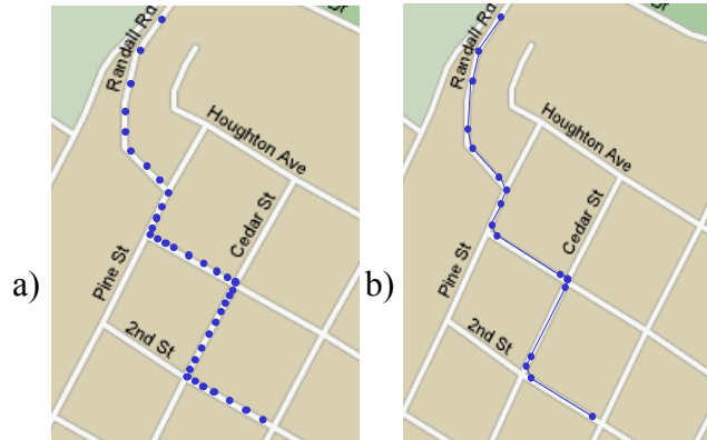
Fig. 2. a) Example roadway network and vehicle position information when sent on a periodic basis. b) Example roadway network with vehicle position information sent only when the trajectory changes significantly.
