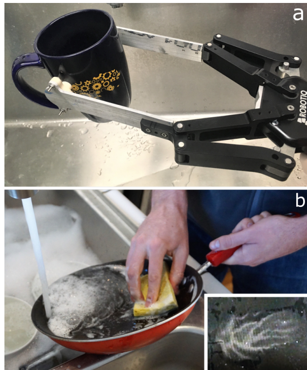
Figure 4.1: Examples of manipulation with lubricated contact – a) The Robotiq gripper picks up a ceramic mug while using a set of soft fingerpads on extended fingertips. The latter of which prevents fluid exposure to electronics. b) Person washes dishes where water, soap and food residue make the pan slippery. Inset: Pressure distribution of a human fingertip that is wrinkly after prolonged exposure to wet conditions, cast in silicone rubber and pressed against the high-resolution tactile sensor developed for [28].
