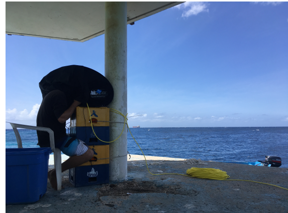
(b) Dr. Rene van der Zande piloting ROV in ergonomic setup with screen cover to reduce sun glare.
