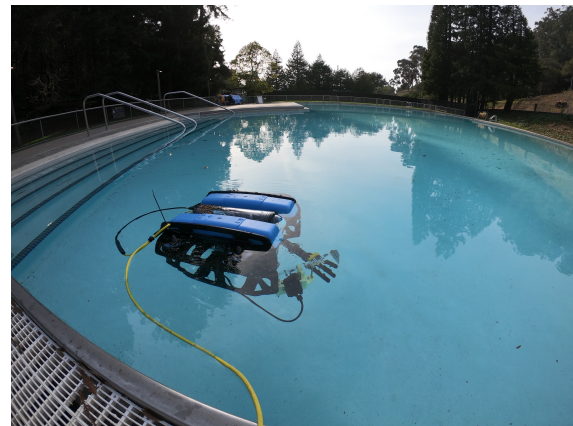
(b) ROV with new end-effectors: impact breaking and toothed gripper.
