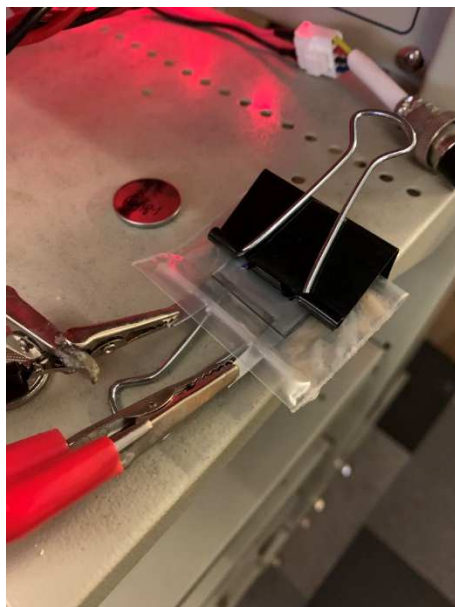
Figure 10. The pouch cell testing platform
