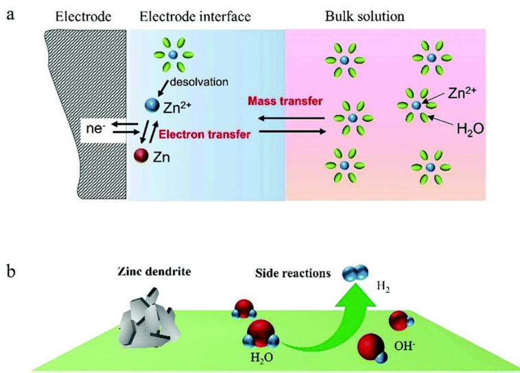
Figure 1. Ideal charge mechanism and real mechanism of aqueous zinc ion batteries from Ref.25
