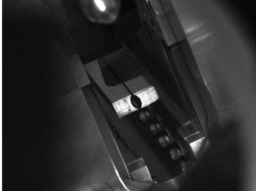
Figure 4.8: Photograph of the entrance to the CPPWG and undulator. The ZnTe crystal used for EOS measurements to optimize THz alignment into the waveguide is currently withdrawn above the beam axis, so that the beam can be transmitted through the waveguide.
