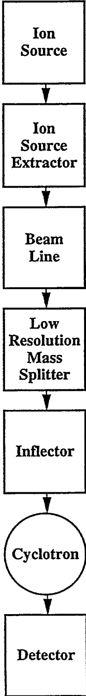
Figure 1. Schematic diagram of the LBL Cyclotron.
