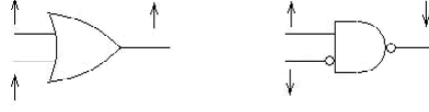
Figure 1: A simple gate consumes maximum instantaneous power when all inputs and outputs take simultaneous transitions.
