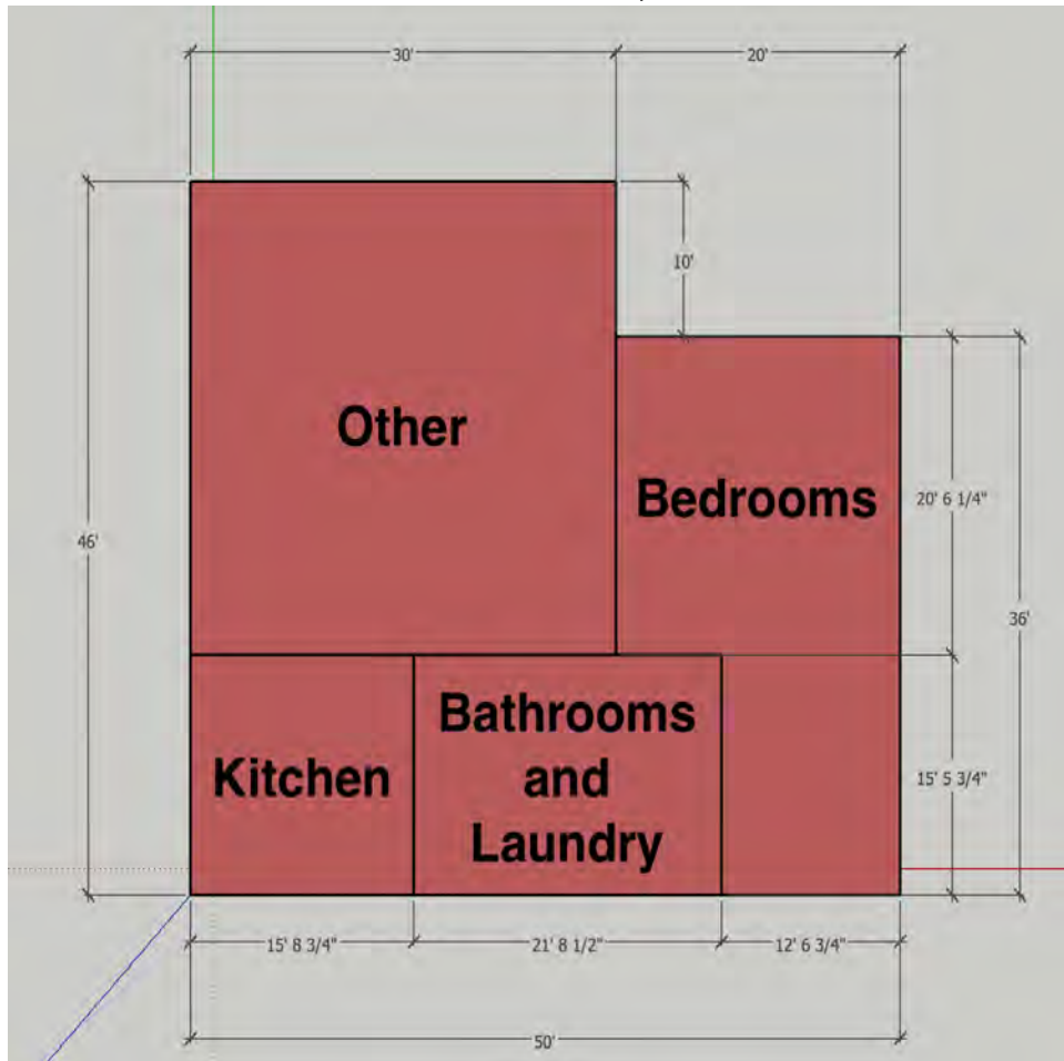
Figure 1: 1-story Single-family Detached Prototype Floor Plan, Includes Zoning And Dimensions. 2,100 ft 2 .
