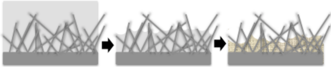
Figure 28: Schematic of nanowire reservoir loading protocol
