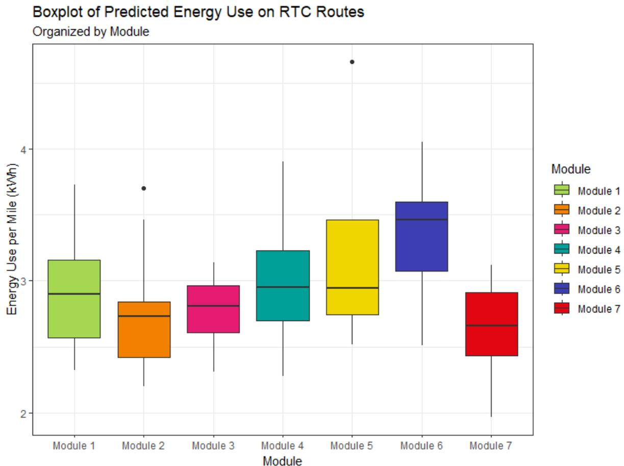
Figure 4: Estimation of energy use on routes for RTP, organized by module. Energy use is presented in kWh/mi (lower is more energy efficient).
