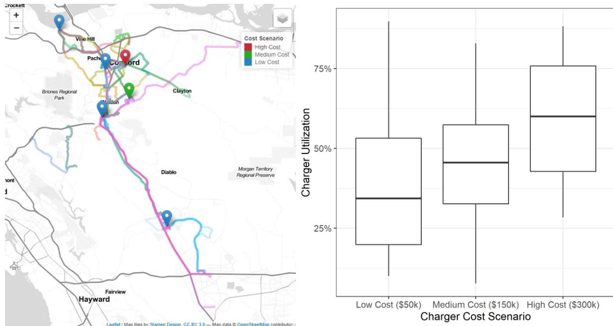
Figure 6: Left: A map of an example network showing the selected locations for charger installation when chargers had a low cost (all colors), a medium cost (red and green locations), and a high cost (red location only). Right: A boxplot of the amount of time opportunity chargers were used in the low, medium, and high-cost scenarios of a previous analysis. Notice that, as the cost of chargers increases, chargers must be used more frequently to be worth their increased cost.
