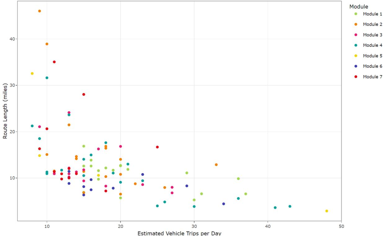
Figure 7: A scatter plot of estimated vehicle trips per day versus the length of the route for all routes in RTP, colored by module. Routes with low length and high frequency (lower left of this chart) are most suitable for electrification.
