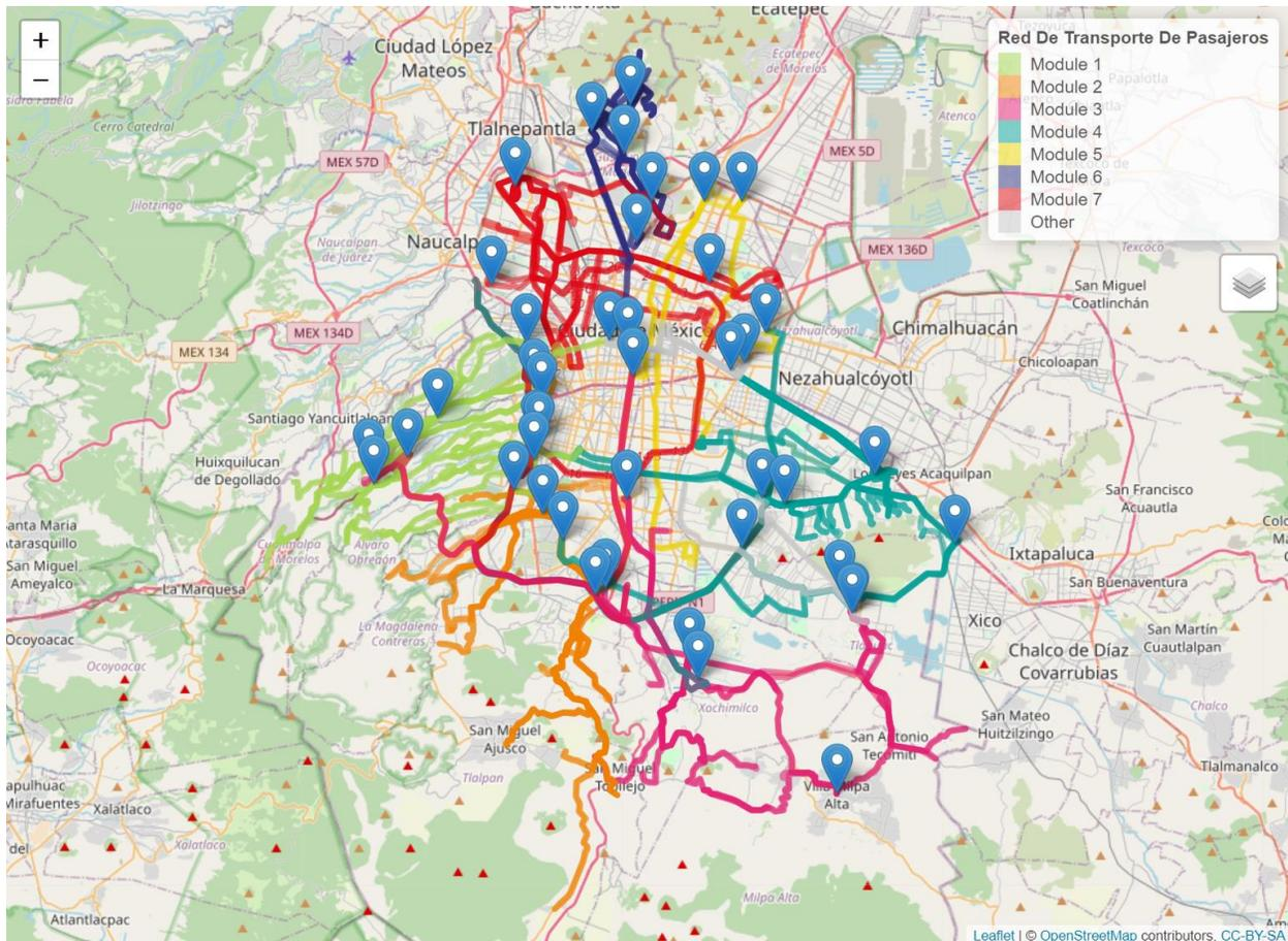
Figure 5: A map of RTP with blue pins identifying stops that are selected as candidate locations for opportunity charging. Routes are colored by module.
