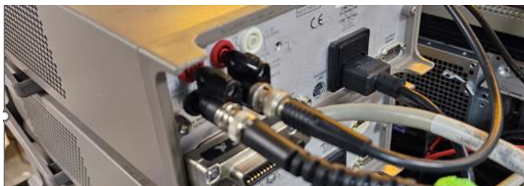
Figure S 35. Picture of the connection to the Keithley 2400 for electrical conductivity measurement.
