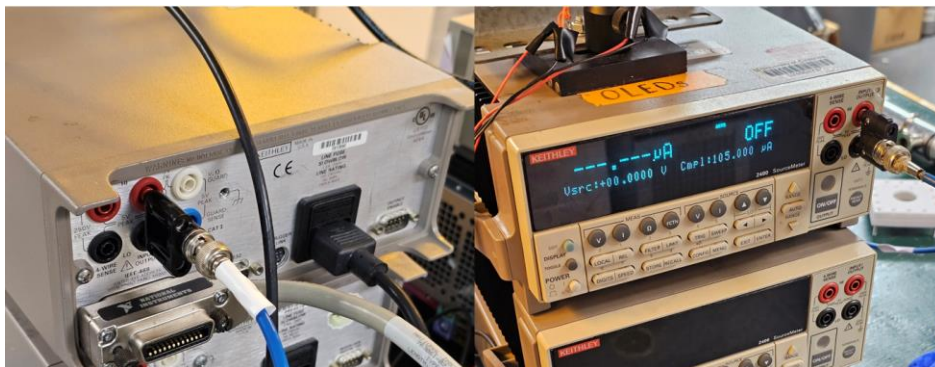
Figure S 31. Locations of the Input/Output connections on the Keithley 2400 to plug the BNC (w/ banana plug) into for Seebeck coefficient measurement.
