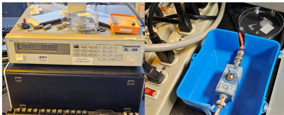
Figure S 32. Picture of the HP663B power supply and the location to connect the BNC cable to the power supply.
