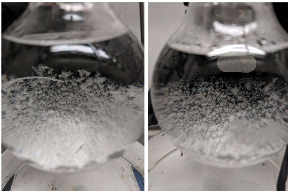
Figure 3.S4. Although it is difficult to visually show, the silanization process using chlorotrimethylsilane (at left) has more points of nucleation than the silanized vials using N,O-bis(trimethylsilyl)acetamide (results at right).
