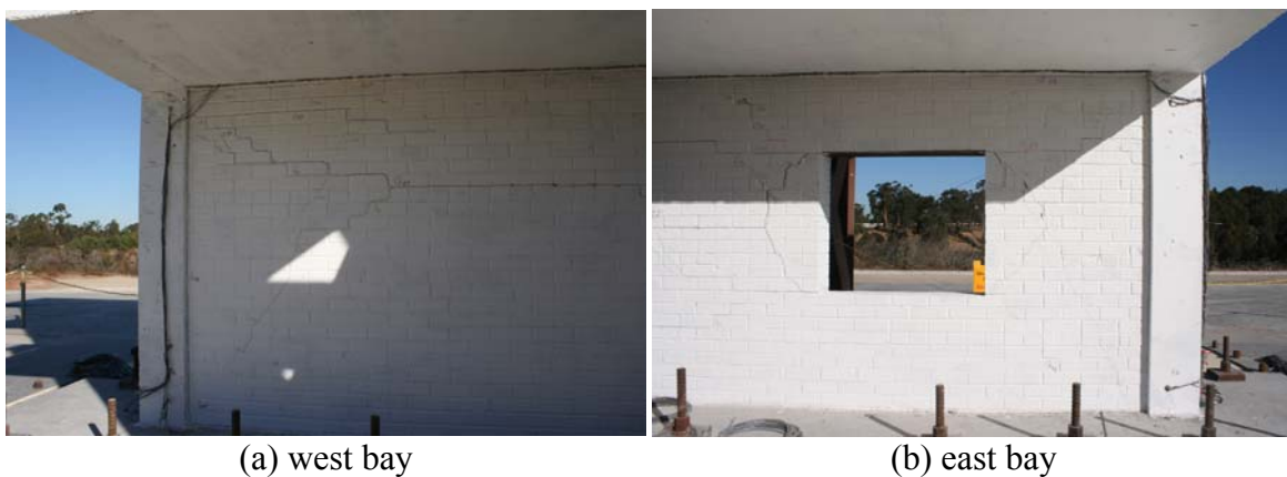
Figure 9.26: Damage in first story after gil100.
