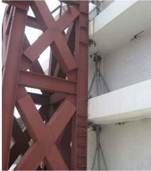
(a) poles used to measure the interstory displacements
