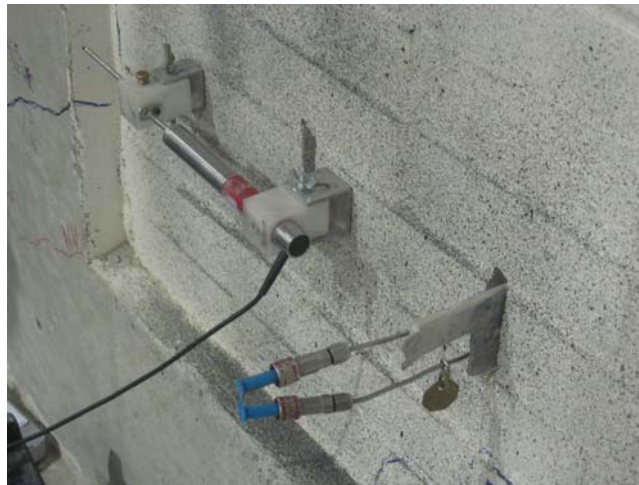
Figure 2.9: Setup for shear tests of existing bed joints exist masonry wall.
