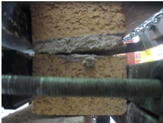
(a) failed mortar-brick
