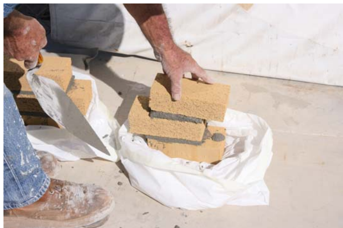
Figure C.30: Building triplet specimens.
