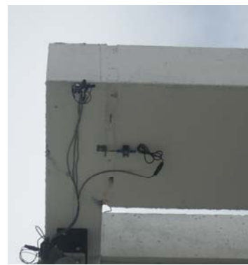
(b) LVDT on the bottom surface
