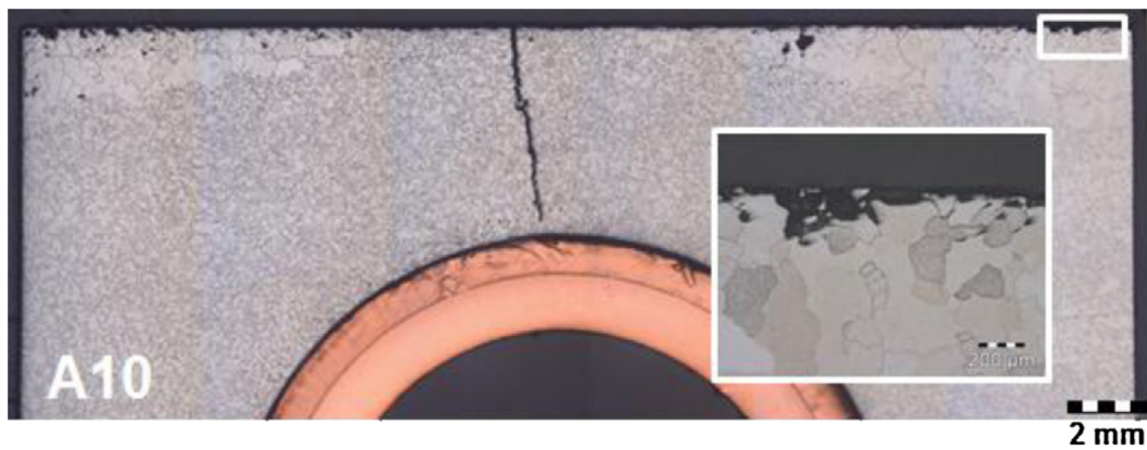
Figure 23: Crack initiation on a tungsten tile from heating face due to residual stresses under high heat flux loading [25].
