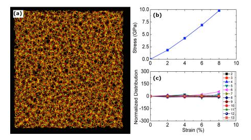
FIG. 1. A bulk silica glass structure simulated under tensile conditions at  $300 \,\mathrm{K}$  and a strain rate of  $2\%/50 \,\mathrm{ps}$  shown in (a), the calculated engineering stress vs. axial engineering strain (b), and associated normalized ring size distributions (c). The number of rings of a given size (n=2, 3,...,12, 13) is also shown in (c). The bulk structure shows negligible ring size variation within the elastic regime of deformation.
