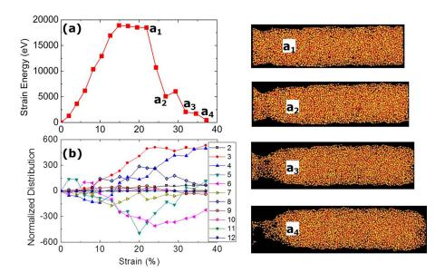
FIG. 5. MD calculated mechanical behavior of a thinner silica glass NW  $(L=14.32\,\mathrm{nm},\,D=5.0\,\mathrm{nm})$  at increasing tensile strains at 300 K. Results show (a) plot of the strain energy variation and (b) the associated normalized ring size distributions as a function of tensile strain. The strain rate is  $2\%/50\,\mathrm{ps}$  as in prior NW simulations. Snapshots reveal particular atomistic morphology at given strain levels during the stretching process of this NW.
