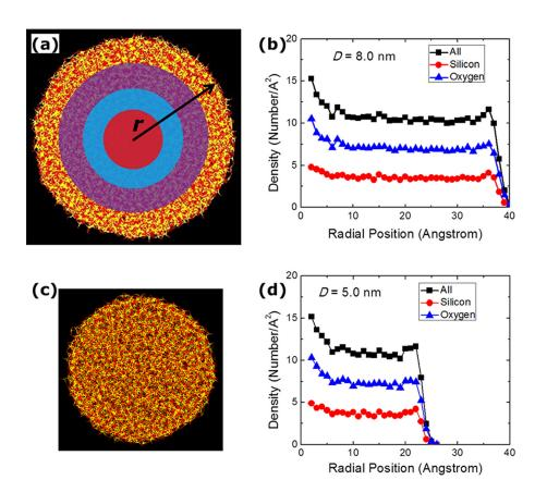
FIG. 2. Radial density distributions of two representative silica nanowires. Figure (a) illustrates how the radial density is calculated for a NW with diameter D=8.0 nm (the radial position starts from the center of the nanowire outwards toward the surface, as shown by the arrow, at increasing distance r). The corresponding radial distribution is shown in (b). Figures (c) and (d) display similar results for another silica NW with smaller D=5.0 nm and corresponding radial density distribution.
