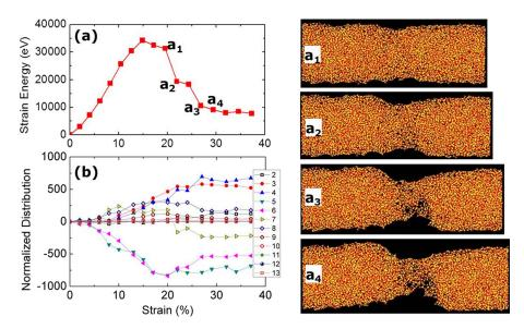
FIG. 4. MD calculated mechanical behavior of a thin silica glass NW  $(L=14.32 \,\mathrm{nm},\ D=6.0 \,\mathrm{nm})$  at varied tensile strains at 300 K. Results show (a) plot of the strain energy variation and (b) the associated normalized ring size distributions as a function of tensile strain. The strain rate remains at  $2\%/50 \,\mathrm{ps}$ . Representative snapshots illustrate the structural evolution and strain levels from the stretching to the breaking stages for this amorphous wire.
