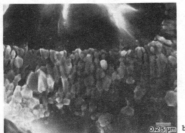
Fig. III-2. SEM fractographs of LBL wire reacted at 700°C/6hours (a) and 700°C/12hours (b). For both heat treatments columnar grains are visible at the Nb/Nb 3 Sn interface. The aspect ratio of the columnar grains decreases with longer heat treatments.
