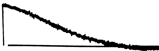
Fig. 2.1. Free induction decay (FID) in the x - y plane.
