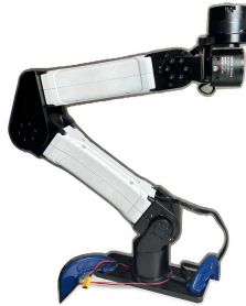
Figure 3.1: The YAM six-DoF manipulator: a low-cost, fixed-base arm with quasi-direct-drive proprioceptive actuators. Joint torques are estimated from motor currents rather than measured by dedicated torque sensors.
