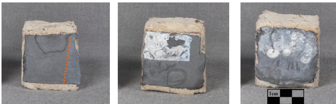
Figure 3 (from left to right) Block 2 following spray application of pure CaLoSiL on the right (see light area, to the right of the red dotted line), and application of CaLoSiL diluted in ethanol (1:1) on the left; block 3 following test application of poultice (white area); and block 8 following brush application of CaLoSiL (visible on bottom of block), followed by the application of ammonium bicarbonate poultice (visible in upper portion) in an attempt to remove the white veil formed. Tidelines are the result of the “Surface Absorption Test” (see Section 5.5.1)
