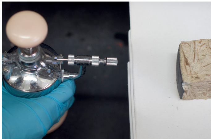
Figure 4: Spray application of the CaLoSiL, on a painted test block, using an atomizer
