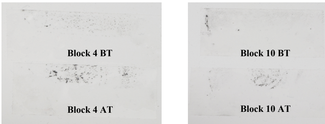
Figure 6 details of the results of the Scotch Tape Tests for two of the blocks, before and after treatment (note: block 4 contains paint without a cactus mucilage binder, while block 10 contains a cactus mucilage binder)
