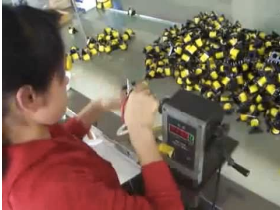
Figure 4.7. Screenshot from YouTube video of Chinese worker assembling transformers.
