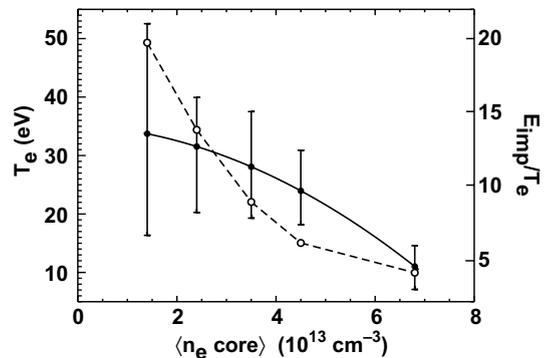
Fig. 5. Comparison of the impact energies inferred from spectral fitting to local  $T_e$  in front of the target. Solid circles are result of parabolic fit to mean  $T_e$  values; open circles represent  $E_{\text{imp}}/T_e$ .
