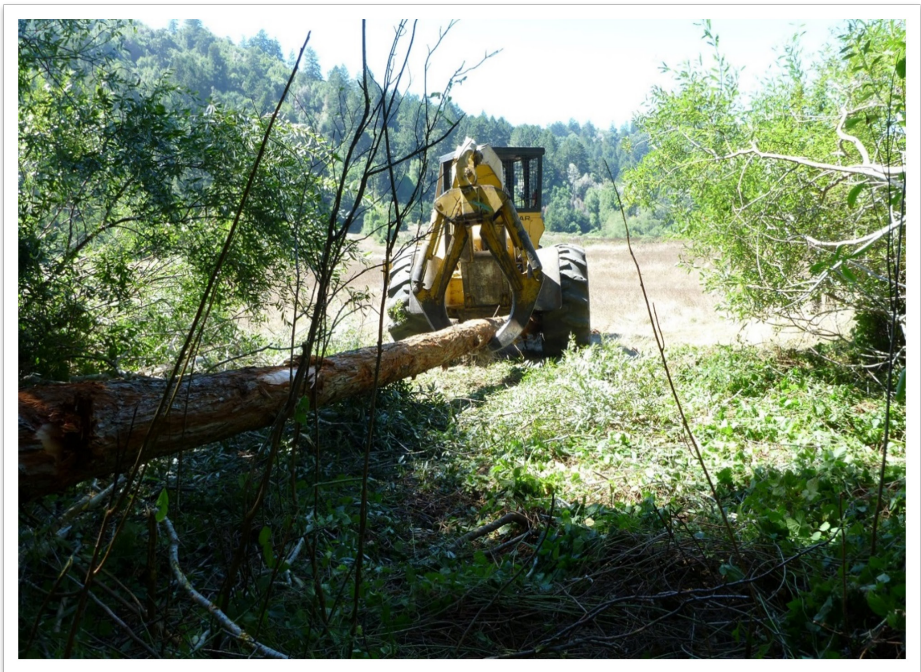
Figure 17. Rubber-tired skidder moving a log. Photo credit: Derek Acomb, CDFW.
