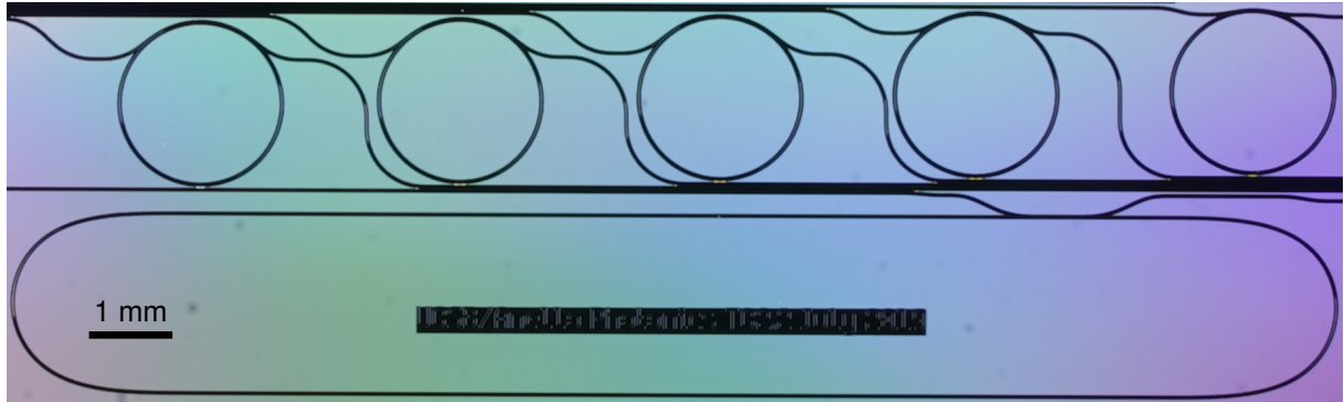
Figure 3.2: Photograph of resonators. Whispering-gallery-mode ring resonators with 1 mm bending radius and 30 GHz FSR, alongside a single-transverse-mode race-track resonator with 1 mm minimum bending radius and 5 GHz FSR. Reproduced from [1].
