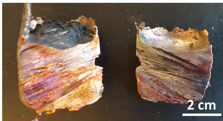
Figure 3-21 Image of a typical as cast Cu-WC nanocomposite ingot by molten salt-assisted incorporation method.
