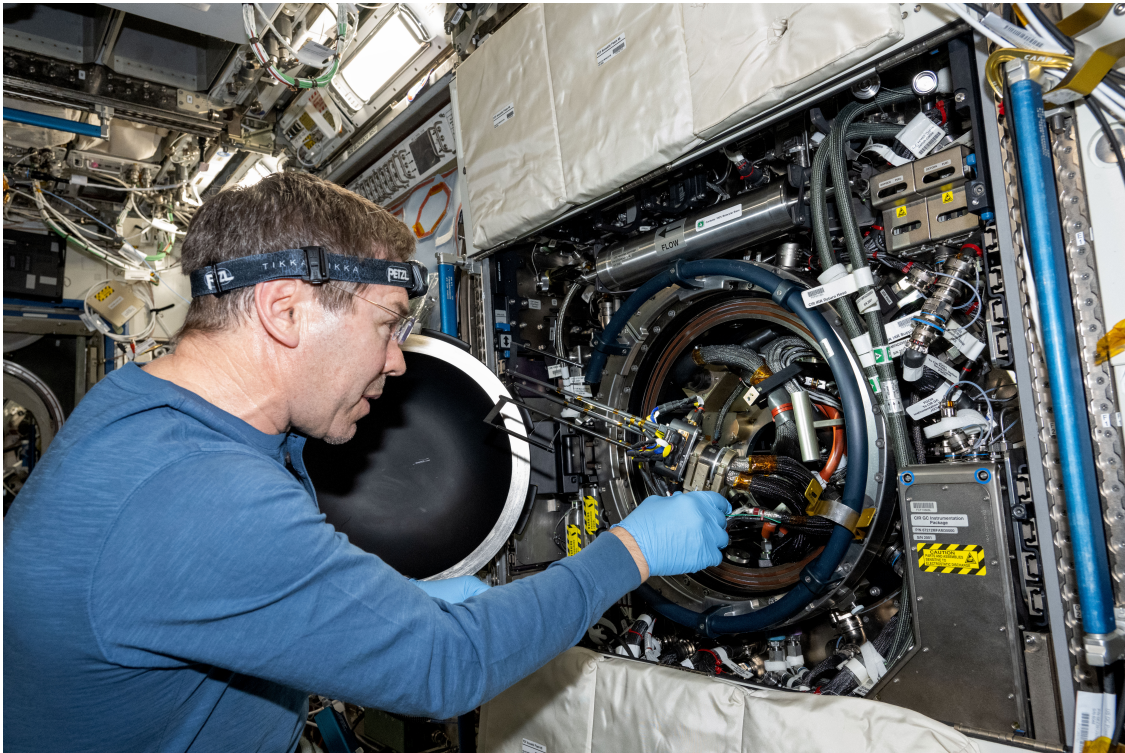
Figure A.2: “Astronaut Mike Barratt replaces fuel bottles inside the Combustion Integrated Rack”. Image by NASA.
