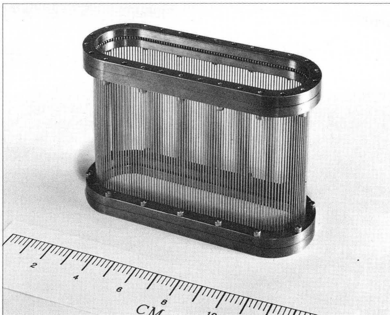
The “birdcage” provides a smooth path for rf fields from the injection straight. The wires are beryllium-copper and 0.46 mm (0.018 in) in diameter.
