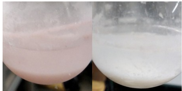
Figure 1. Images characterizing samples at two stages of the low-temperature synthesis as \text{Ir}(\text{CO})_2(\text{acac}) reacted with zeolite HY to give a loading of 1.0 wt% Ir. Left: a After \text{Ir}(\text{CO})_2(\text{acac}) and zeolite HY had been slurried in n -pentane for 24 h in a dry ice bath at (193 K); right: after the slurry had been allowed to warm to 298 K in a period of approximately 30 min.
