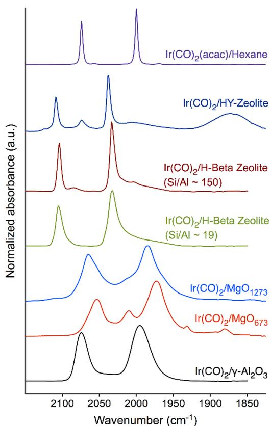
**Figure 2.** IR spectra in the  $\nu_{\text{CO}}$  region of supported  $\text{Ir}(\text{CO})_2$  complexes demonstrating the variation FWHM as the uniformity of the bonding sites on the support surfaces decrease, roughly from top to bottom. The  $\text{Ir}(\text{CO})_2/\gamma\text{-Al}_2\text{O}_3$  is taken from the work of Lu et al.<sup>13</sup>
