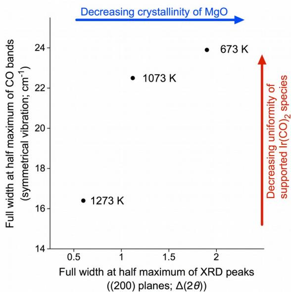
**Figure 3.** Correlation between the degree of crystallinity of the MgO support as measured by the FWHM of the MgO (200) plane determined by XRD measurements and the degree of uniformity of the MgO-supported  $\text{Ir}(\text{CO})_2$  complexes measured by the FWHM of the symmetric
