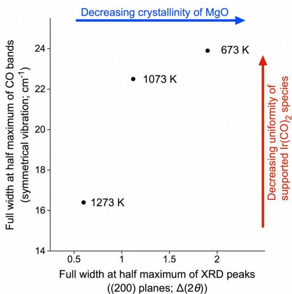
**Figure 3.** Correlation between the degree of crystallinity of the MgO support as measured by XRD and the degree of uniformity of the MgO-supported Ir(CO)<sub>2</sub> complexes measured by the FWHM of the symmetric CO stretching band determined by IR spectroscopy. Temperatures next to the data points represent the pretreatment temperature of the MgO support.
