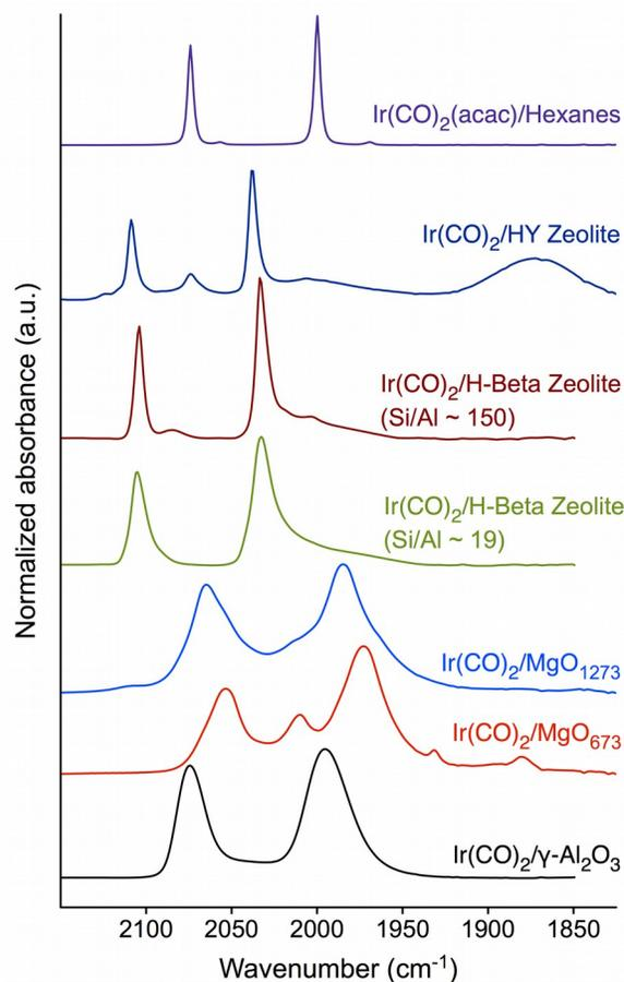
**Figure 2.** IR spectra in the  $\nu_{\text{CO}}$  region of supported  $\text{Ir}(\text{CO})_2$  complexes demonstrating the variation FWHM as the uniformity of the bonding sites on the support surfaces decreases, roughly from top to bottom.  $\text{Ir}(\text{CO})_2$  on HY zeolite was made by the low-temperature method described in the text. The spectrum of  $\text{Ir}(\text{CO})_2/\gamma\text{-Al}_2\text{O}_3$  is taken reproduced from the work of Lu et al.<sup>19</sup>
