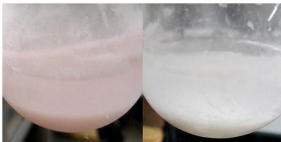
**Figure 1.** Images characterizing samples at two stages of synthesis as Ir(CO)<sub>2</sub>(acac) reacted with zeolite HY to give a loading of 1.0 wt% Ir. Left: After Ir(CO)<sub>2</sub>(acac) and zeolite HY had been slurried in *n*-pentane for 24 h in a dry ice bath (193 K); right: after the slurry had been allowed to warm to 298 K in approximately 30 min.
