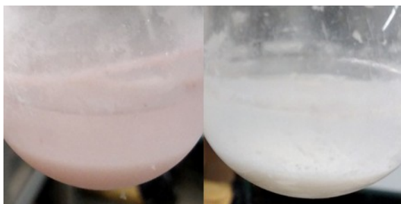
Figure 1. Images characterizing samples at two stages of synthesis as Ir(CO) 2 (acac) reacted with zeolite HY to give a loading of 1.0 wt% Ir. Left: After Ir(CO) 2 (acac) and zeolite HY had been slurried in n -pentane for 24 h in a dry ice bath (193 K); right: after the slurry had been allowed to warm to 298 K in approximately 30 min.
