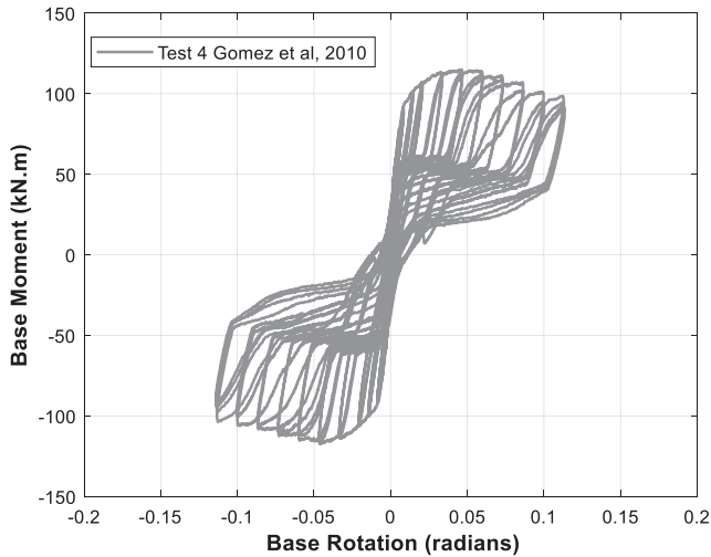
Fig. 6. Experimental hysteresis curve of a typical Design Guide 1 CBC (Gomez et al. [8]).
