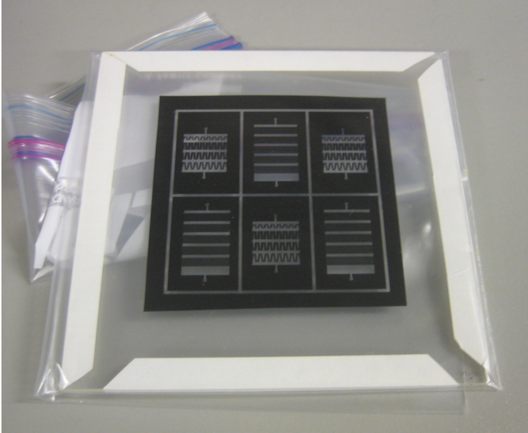
Figure 4.1.2: Microfluidic photolithography mask showing 6 separate chambers created by mounting a printed transparency design onto a 4" by 4" optical grade borosilicate glass
