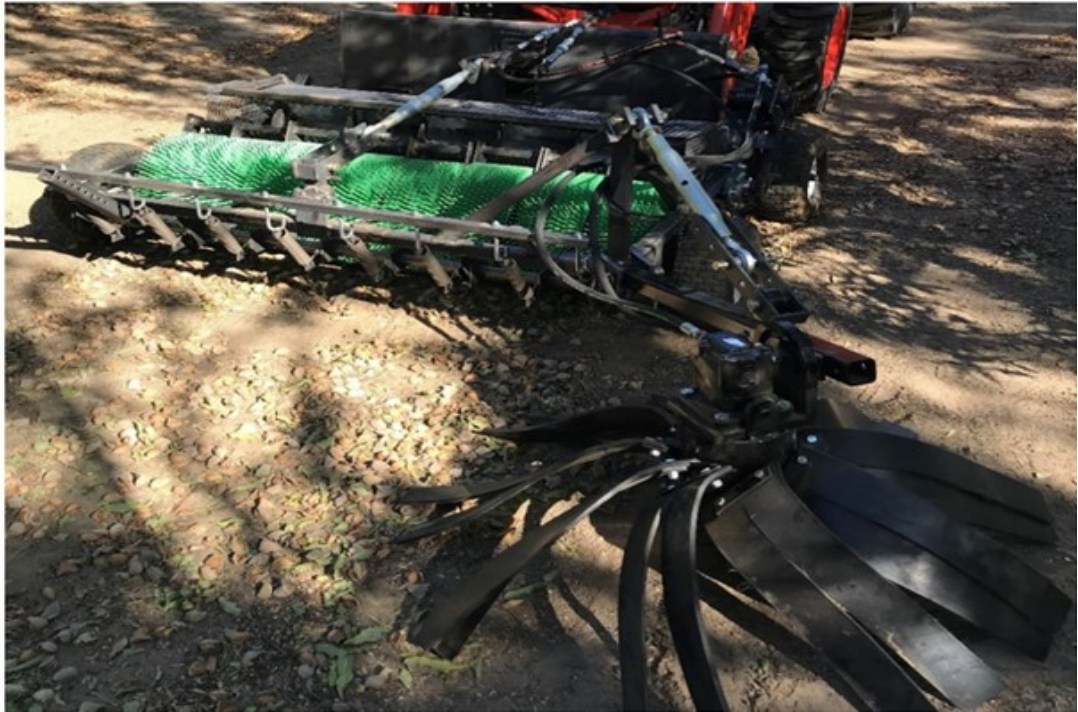
Figure 2.4: Second design with low-speed rubber brush
