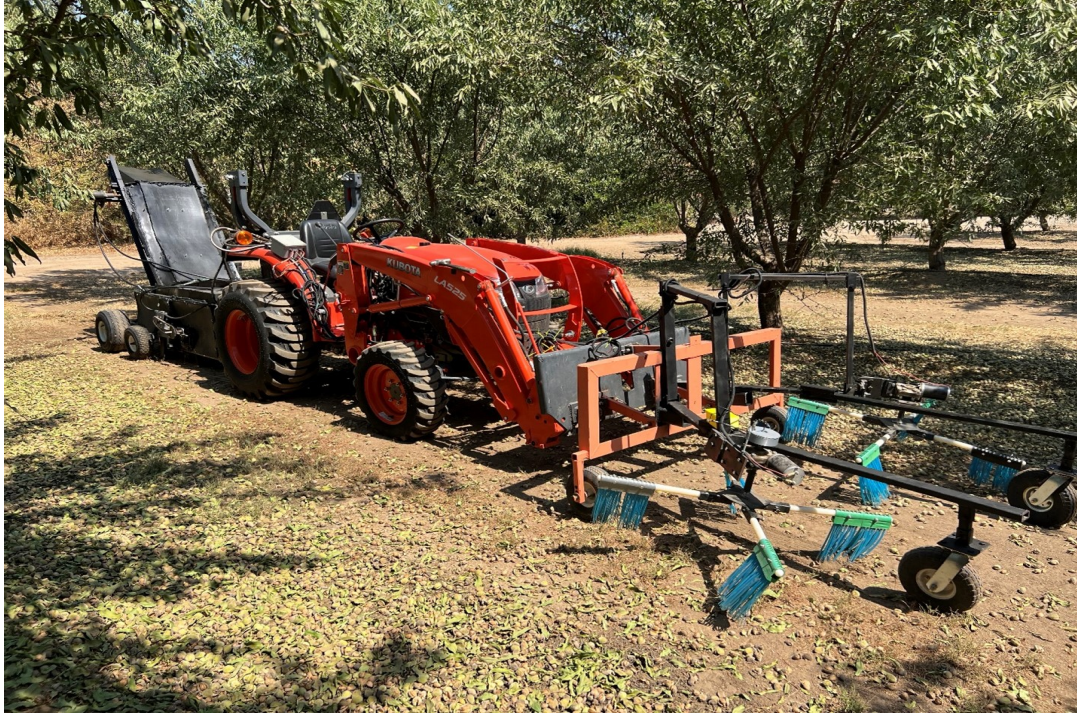
Figure 2.10: Final prototype of the almond pickup system with integrated sweeping mechanism
