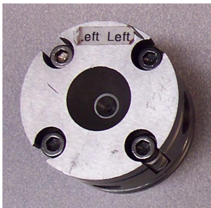
Figure A.5: Symmetric diamond anvil cell. The screws labeled "Left" are those that are reverse threaded.
