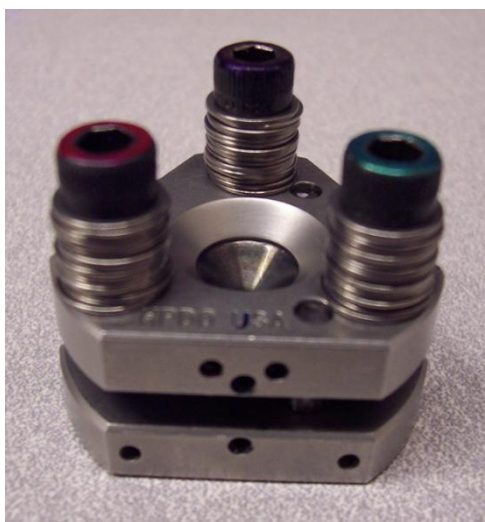
Figure A.3: A Merrill Bassett cell from High Pressure Diamond Optics in Tucson, Arizona.
