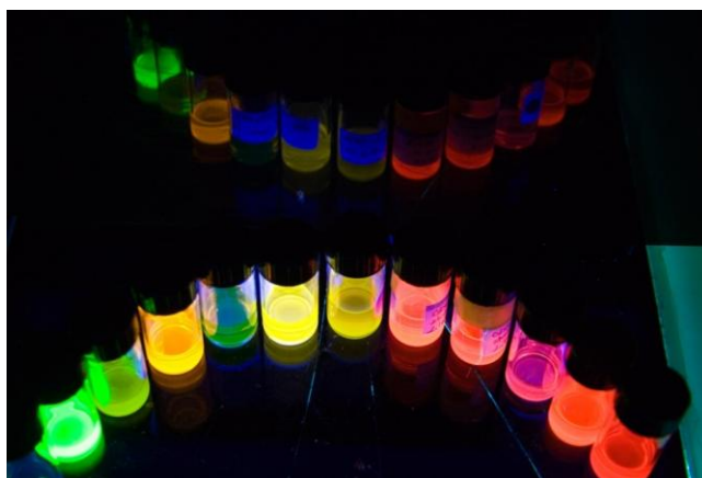
Figure 1.3: Photograph of the fluorescence from cadmium selenide nanocrystals of different sizes. Particles shown here were synthesized by Jennifer Dionne and the author.
