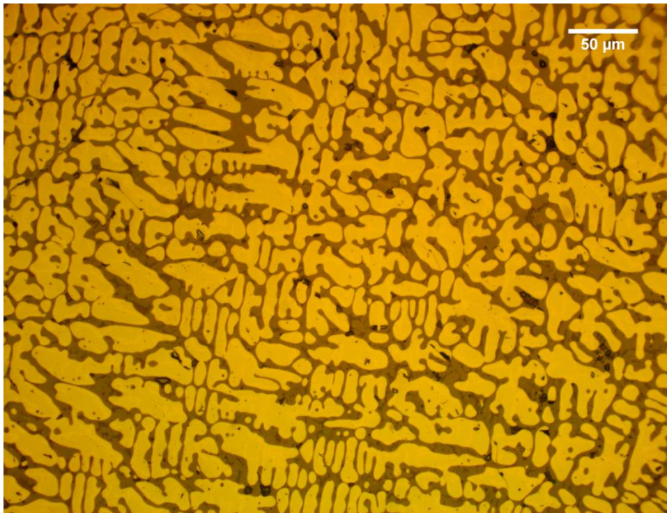
Figure II2e. Primary wüstite
