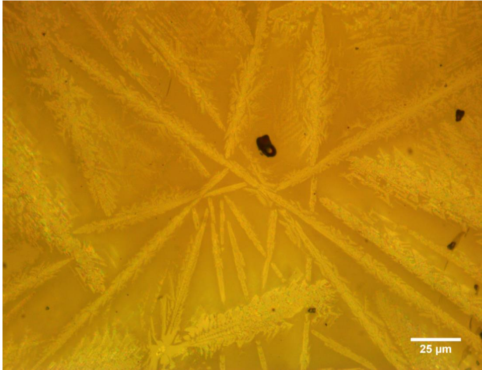
Figure II3j. Optical micrograph of spinifex microstructure
