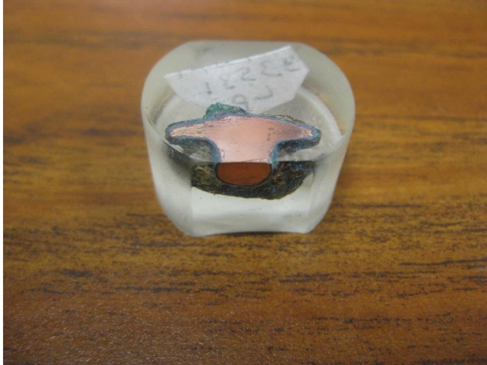
Figure III11b. Mounted with double cross section for analysis of both head and shank, cracks on top of head are visible to naked eye
