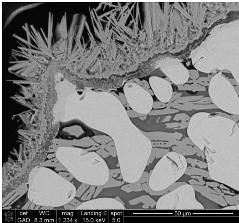
Figure III1g. Backscattered micrograph of phases and external prilly slag surface
