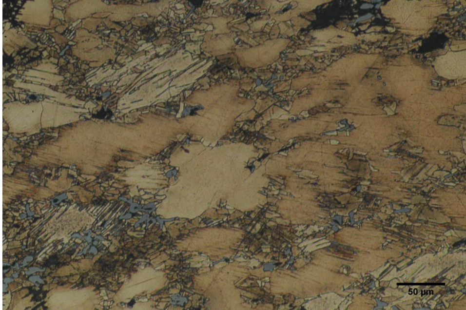
Figure III9b. Optical micrograph showing phase differentiation, sulphidic green zinc blotches, and strain lines, etched with ferric chloride
