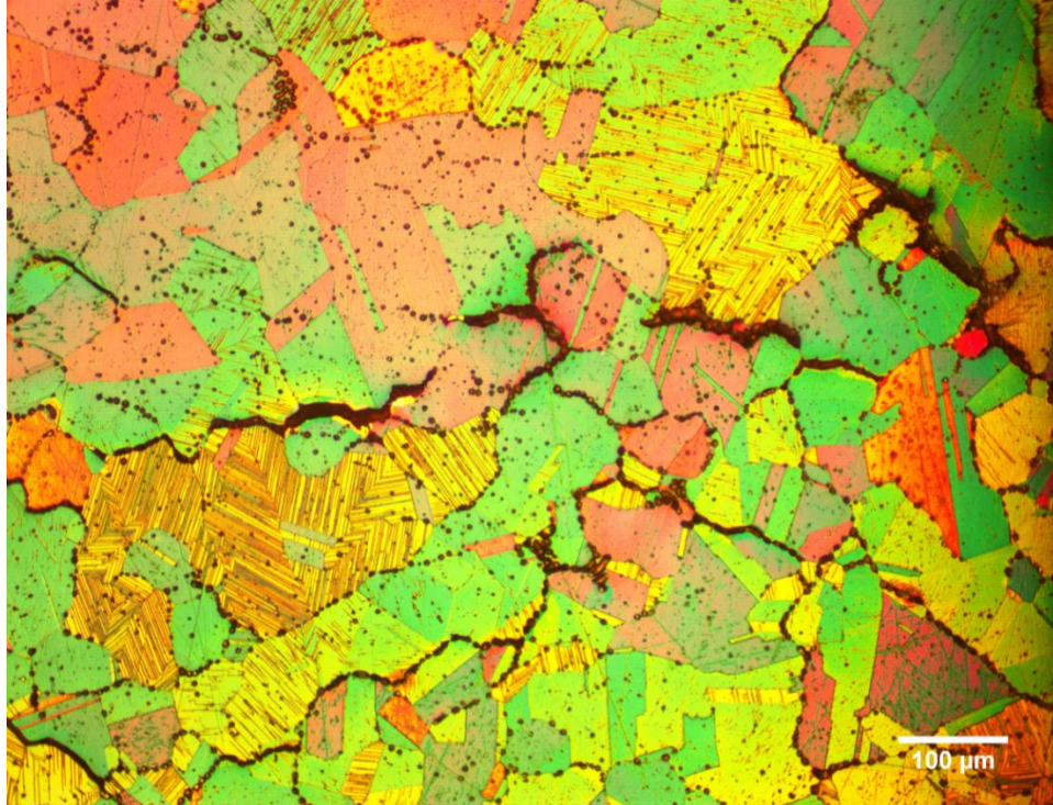
Figure III11f. Peculiar geometric microstructure in shank
