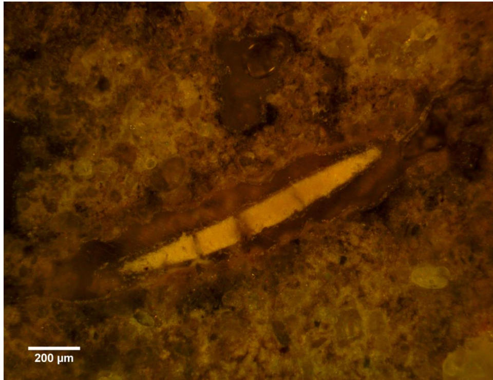
Figure II5b. Polarized optical micrograph of shell embedded in detritus
