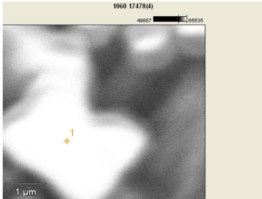
Figure I53f. EDS in wt% (excluding 0.04Sc) 47.06Fe 0.23Ti 2.14Ca 1.57K 10.80Si 1.44Al 0.73Mg 35.99O
