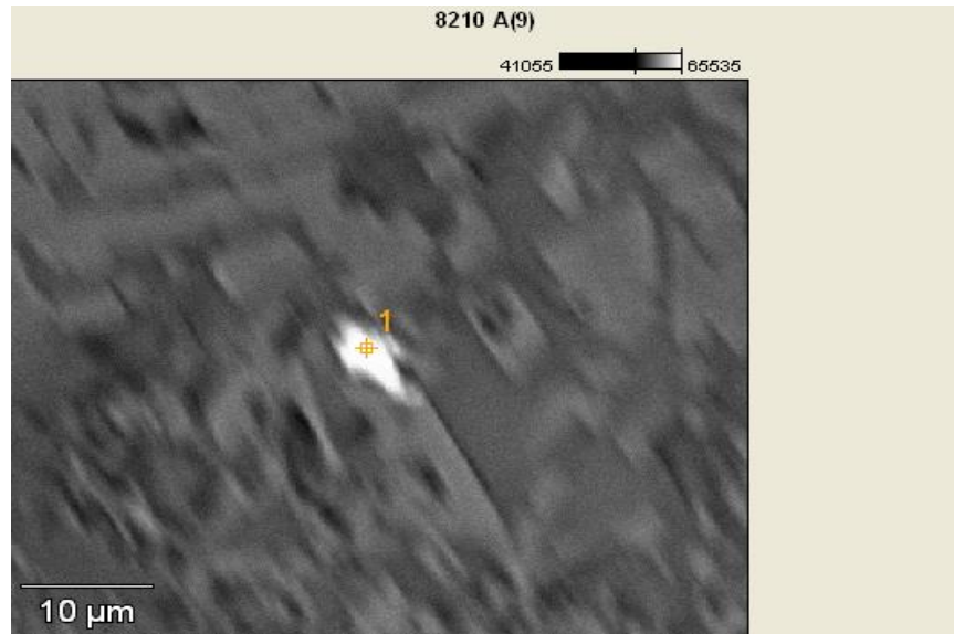
Figure II5f. EDS in wt% of major metal constituents: 9.33Cu 3.18Ni 2.90Zn 13.55Fe
