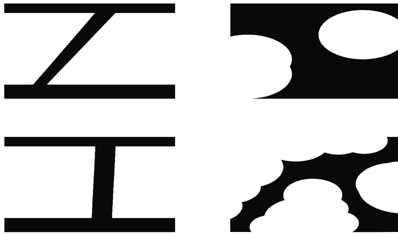
Figure 2.8. The initial conditions used for the softening (top left), stiffening (top right), softening to stiffening (bottom left) and stiffening to softening (bottom right) optimizations. The boundary conditions imposed on the softening, stiffening, and softening to stiffening cases are: 1) fixed along the top edge, 2) roller along the bottom edge, and 3) applied displacement along the lower right edge. The boundary conditions imposed on the stiffening to softening case are: 1) fixed along the left edge and the top right corner, 2) roller along the bottom edge, and 3) applied displacement along the lower right edge.
