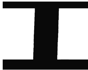
Figure 2.10. The initial condition used for the cubic sweep ratio 20 optimization. The boundary conditions imposed are: 1) fixed along the top edge, 2) roller along the bottom edge, and 3) applied displacement along the lower right edge.
