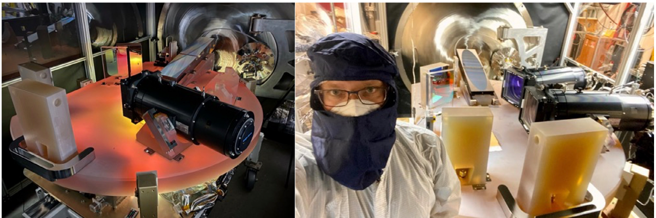
FIGURE 3 Left: Keck Planet Finder illuminated from underneath showing subsystems delivered during AIT in November 2022 by Jerry Edelstein. Right: PI Andrew Howard next to the fully populated optics bench and vacuum chamber May 2022.
