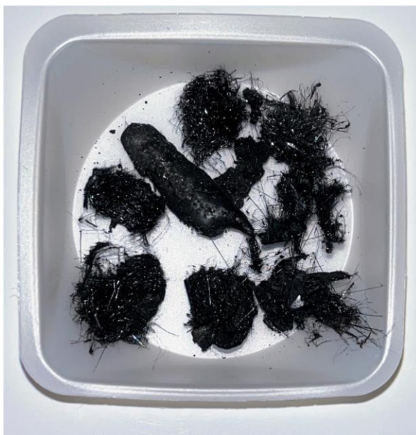
Fig. 2.1: NbS 3 material synthesized by CVT method. The bulk crystal material was provided by the collaborators at the University of Georgia.
