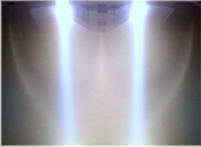
Fig. 2. Photographs of light emission in the drift space for the case of grounded target. The bias potential is about zero.
