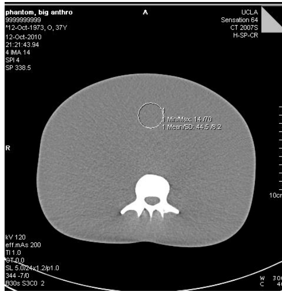
Figure 9.5 ROI in a homogeneous area in thorax phantom for the benchmark between simulated images and actual images.
