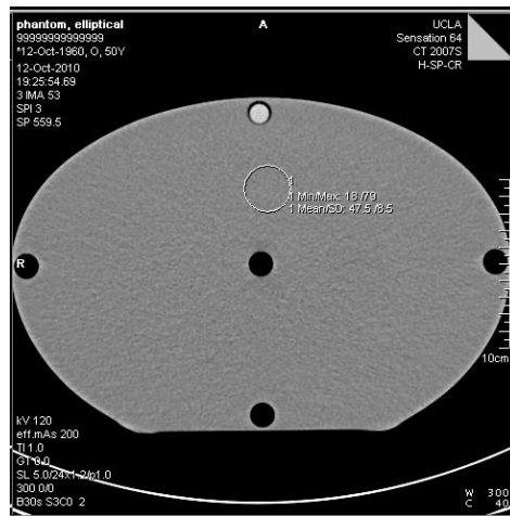
Figure 9.4 ROI in the elliptical phantom for the benchmark between simulated images and actual images.
