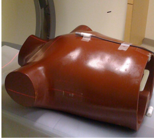
Figure 8.8 The setup of the experiment: a Radcal small ionization chamber was placed on the anterior surface of an anthropomorphic thorax phantom.
