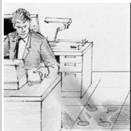
FIGURE 2 Underfloor air distribution can provide building occupants with control over temperature and air flow. (Image: Tate Access Floors)
